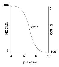
Given: The above graph Find: What is the most effective pH range for dosing chlorine Since HOCl is 2 orders of magnitude more effective than OCl<sup>-</sup>, **the most effective pH would be towards the acidic end** Note: There is a problem with corrosion at the acidic pHs
